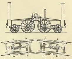
Fig. 5 .- " South Carolina," 1831, and Plan of its Running Gear.
