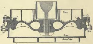
Fig. 50.-Mould and Flask in which Wheels are Cast.
