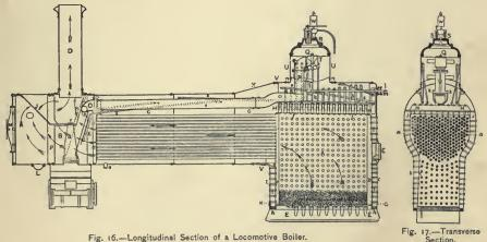
the chimney D. The fire-box and tubes are all surrounded with water, so that as much surface as possible is exposed to the action of the fire. This is essential on account of the large amount of water which must be evaporated in such boilers. To create a strong draught, the steam which is exhausted from the cylinders is discharged up the chimney through pipes, and escapes at e.
