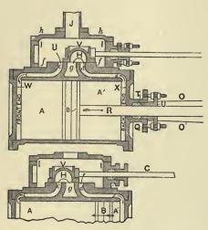
Figs. 20 (above) and 21.—Sections of a Locomotive Cylinder.
