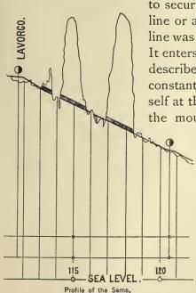
to secure a longer distance than a straight line or an ordinary curve would give; the line was therefore doubly curved upon itself. It enters the mountain at a high elevation, describes a circle through the rock and, constantly descending, reappears under itself at the side; still descending, it enters the mountain at another point and con-
