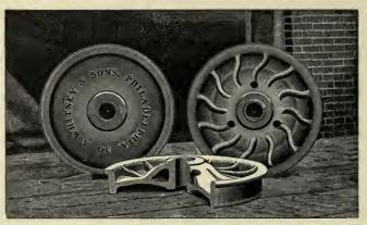
Fig. 51 -Cast-iron Car Wheels.
