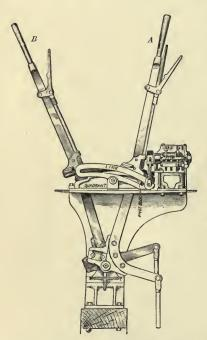
Section of Saxby & Farmer Interlocking Machine. (Showing two levers and locking mechanism. A is normal, B is reversed.)
