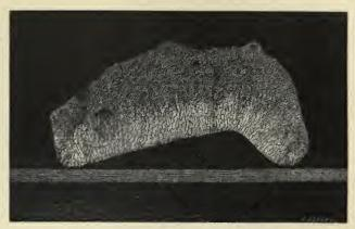
Fig. 52.-Section of the Tread and Fiange of a Car Wheel.
