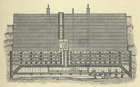
Transverse Section of Pneumatic Caisson.
