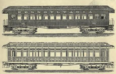
Fig. 54.-Modern Passenger-car and Frame.
