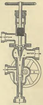
Fig. 19.—Injector used on Locomotives.
