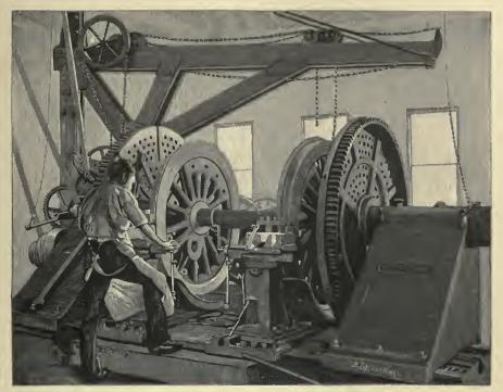
Fig. 25.—Turning Locomotive Tires.
