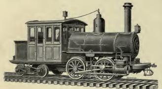
Fig. 32.—"Forney" Tank Locomotive. By the Rogers Locomotive and Machine Works, Paterson, N. J.
