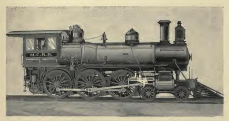
Fig. 28.—Ten-wheeled Passanger Locomotive. By the Schenectady Locomotive Works.
