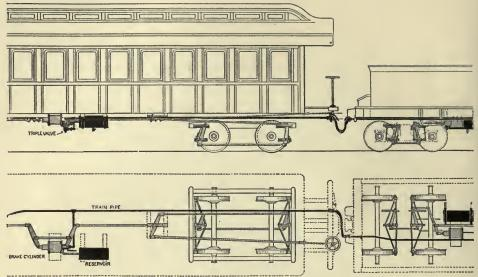
Plan and Elevation of Air-brake Apparatus.-Reser-
