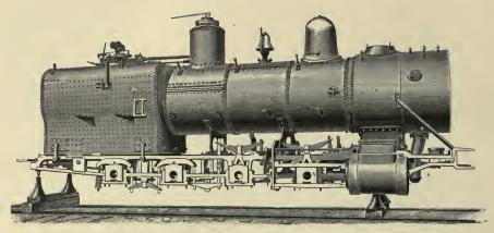
Fig. 29.-Consolidation Locomotive (unfinished).
