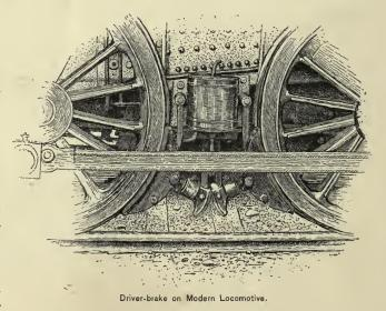
raised the piston, which through a lever and rod raised the togglejoint between the brake-blocks and forced them against the treads of the wheels. Essentially the same method of applying the retarding force can now be seen on most passenger engines, and often, but not so commonly, on engines for freight service. For
